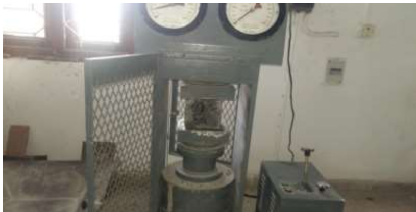
Figure2: set up for compressive strength test
