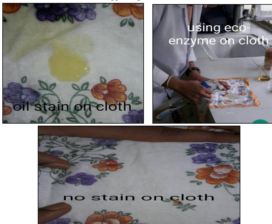
Fig.4. Removal of stain on clothing material using synthesized Eco-Enzyme.
