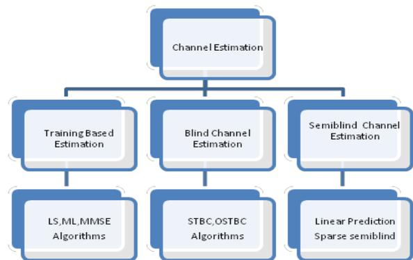
Figure 2: classification channel estimation algorithms
