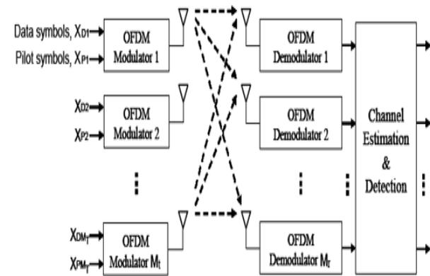
Figure1: Typical MIMO system Model.
