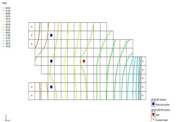
Figure 2. Head distribution during steady pumping
